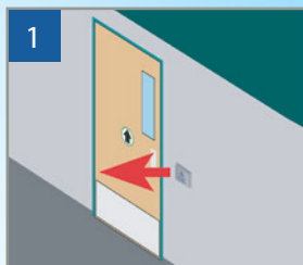
1 Remove existing touch push plate and disconnect the two (2) existing in-wall wires from the push plate and door control activation.
