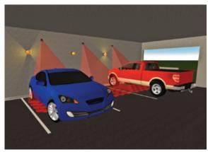
INFRARED PRESENCE DETECTION Detects when an object is too close to a wall or occupying a space
