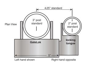
The IDC GL160 and 260 series electromechanical GateLoks are designed to provide access control and remote locking and unlocking capability for manual or automatic chain link, tubular steel and wrought iron sliding or swinging gates.
