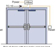
Pair of doors with two locks and required TC-3 cable for power and slave operation Pushing either door triggers the delayed release of both doors.
