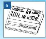
Install the 900 MHz wireless receiver in the header (solo separately).
